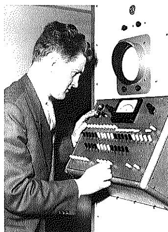
ZEBRA Operator Panel. The small scope showed the contents of accumulators and counters in binary form, suitable to follow the progress of the program execution
