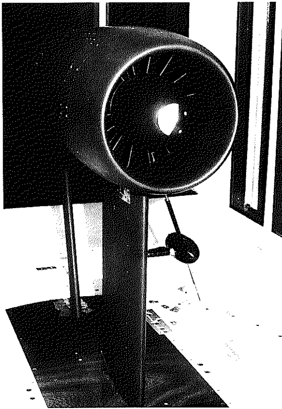
A wind tunnel model for basic studies of the Fan Noise of a High By-pass Jet Engine
