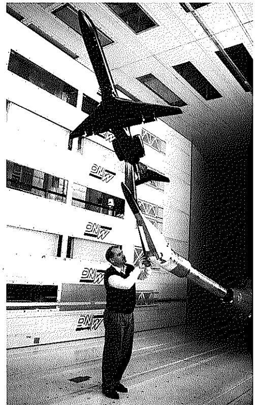
Deep-stall test of the Fokker 130 in the DNW
