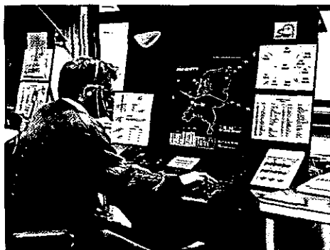
Air traffic controller working position of the NLR ATC Research Simulator (NARSIM)
