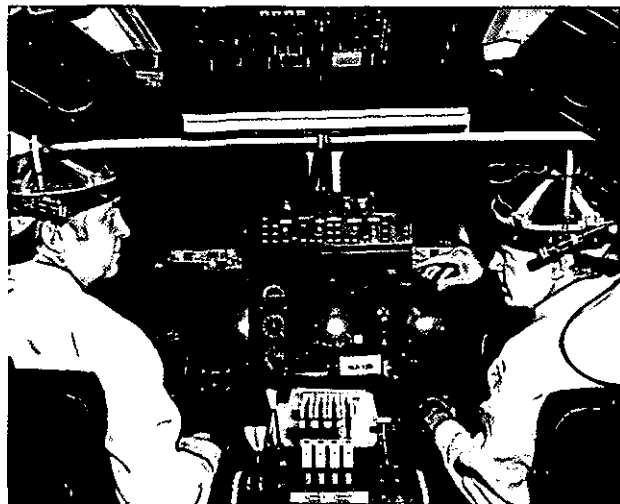
One of the crews, equipped with miniature video cameras for head tracking in NLR's Research Flight Simulator, participating in a collaboration with the FAA
