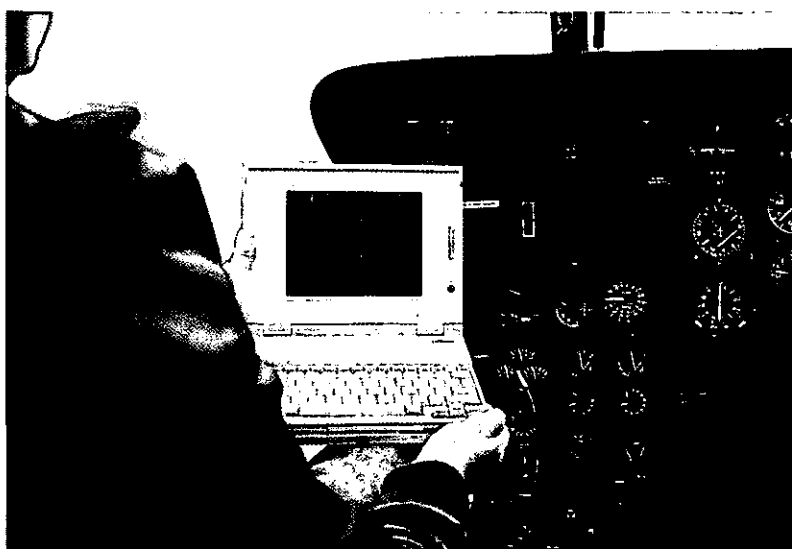
Test of Moving Map in BO 105C helicopter of the national police (Rijkspolitie)
