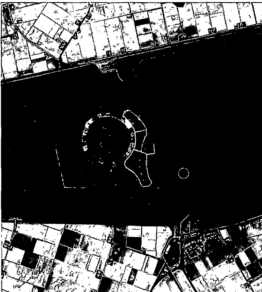
Remote sensing image showing dredgings storage and water flow phenomena in Ketelmeer, the Netherlands (Image by SPOT satellite, 10 m resolution)
