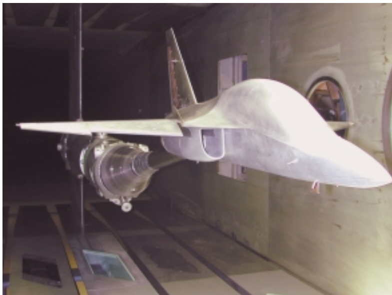
AerMacchi AEM/YAK 130 model in the DNW-HST wind tunnel
