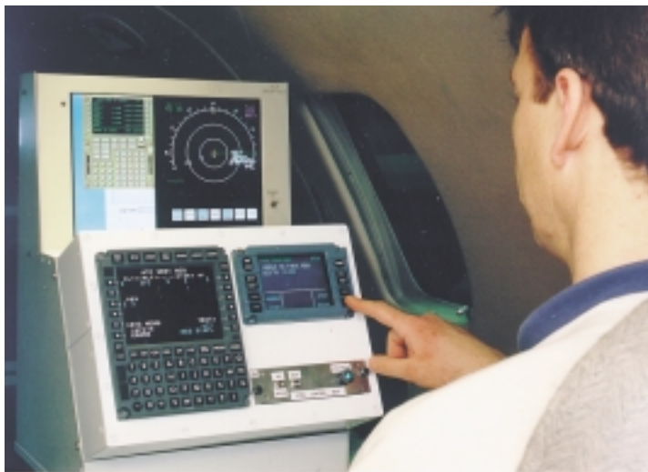
Testing an Air-Ground Digital Datalink in the Cessna Citation II research aircraft of NLR, in a European collaboration
