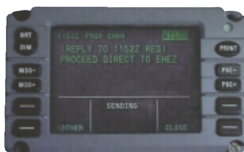
Controller-Pilot Datalink Communications in the EOLIA ProATN programmes: Pilot request and ATC clearance
