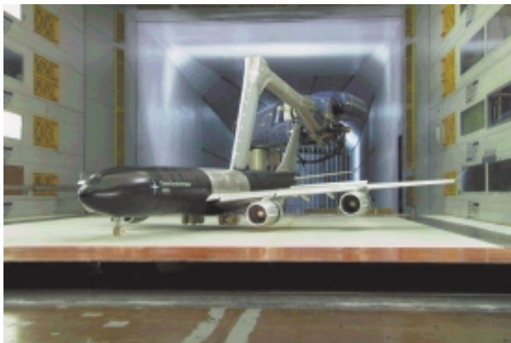
Airbus A340-500/600 model in the reverse thrust configuration, with a moving belt ground plane for the simulation of ground effects
