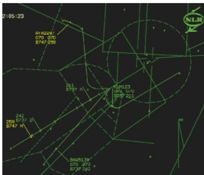
Preliminary ATC display tool that depicts on the extended centre line of the runway the positions of aircraft on Continuous Descent Approach paths
