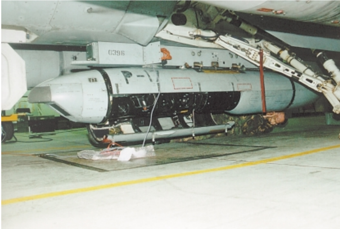
Installation of ORPHEUS with OMID interface on an F-16 MLU
