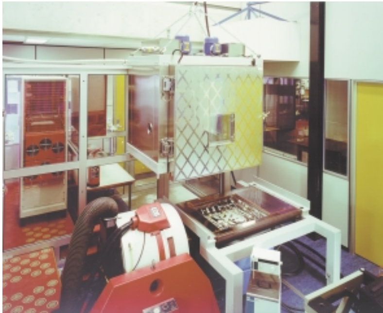
Vibration and Shock Test facility with thermal chamber
