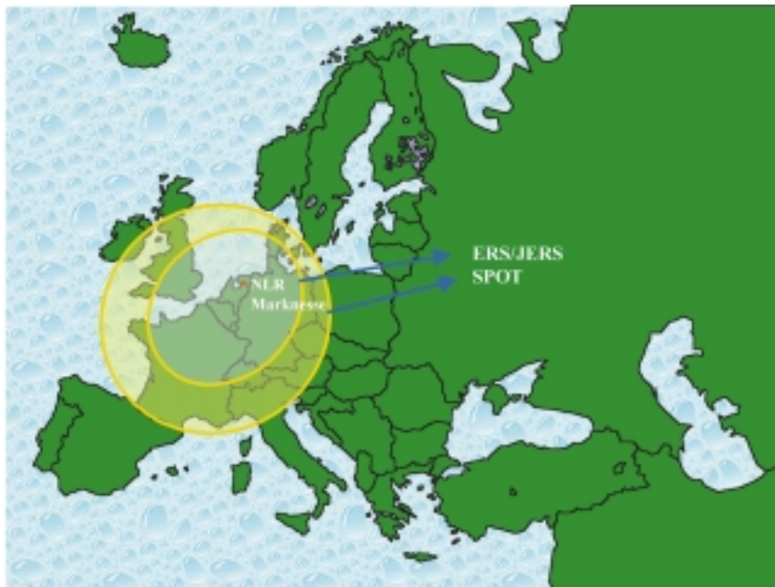
Fig. 2 – Spatial coverage (footprint) of ERS and SPOT satellites received by RAPIDS deployed at NLR-NOP
