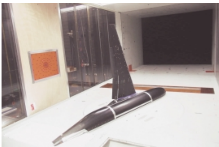
Acoustic measurements on a semi-span model in the DNW-LST
