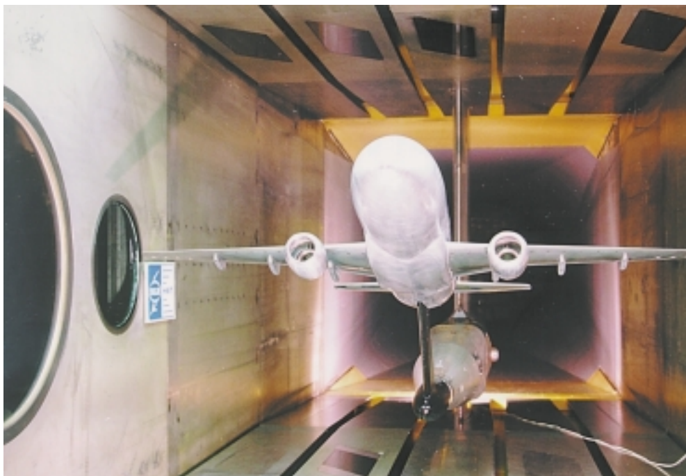
Dornier 728 model in DNW-HST wind tunnel
