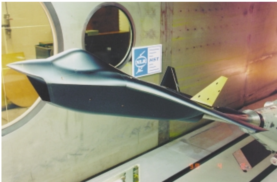
Model of the Boeing Joint Strike Fighter, possible successor of the F-16 of the RNLAf, in the DNW-HST wind tunnel at NLR Amsterdam
