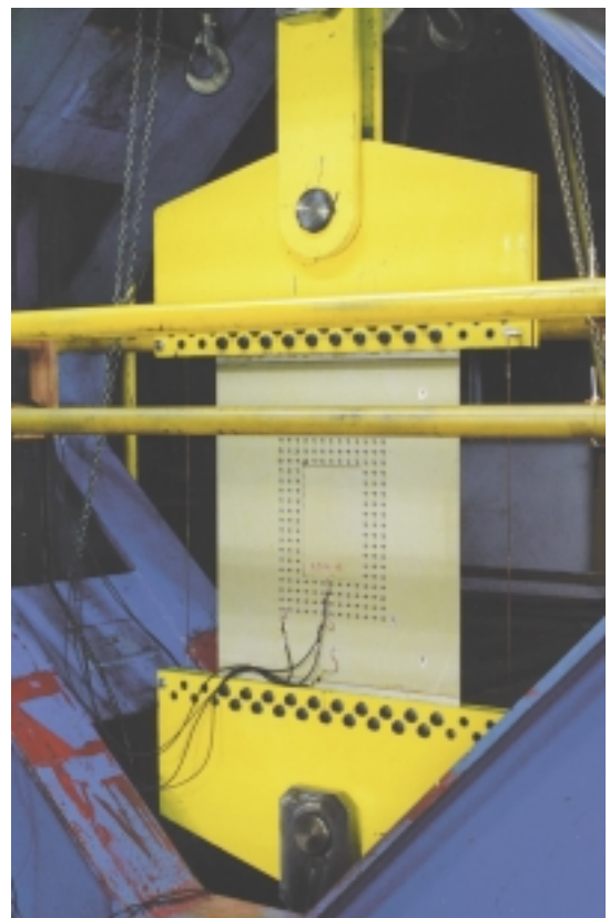
Tension test on repaired GLARE panel
