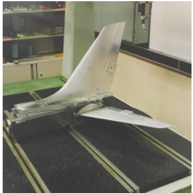
Tail part of a Dornier 728 low-speed model, equipped with an adjustable stabilizer and remote controlled rudders and elevators
