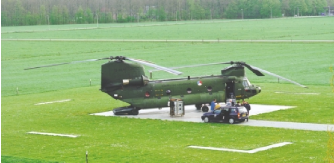
EMC test on a Chinook helicopter at the Open Area Test site
