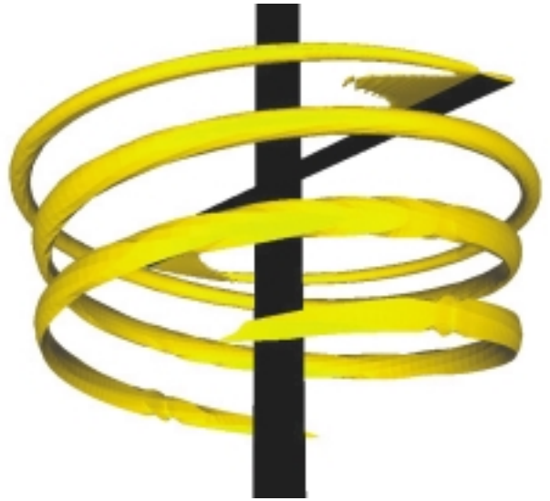
Tip vortex of helicopter in hover computed with Euler method
