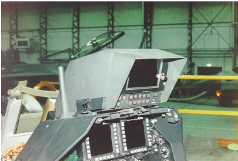
Lockheed Martin F-16 MLU flight test display console
