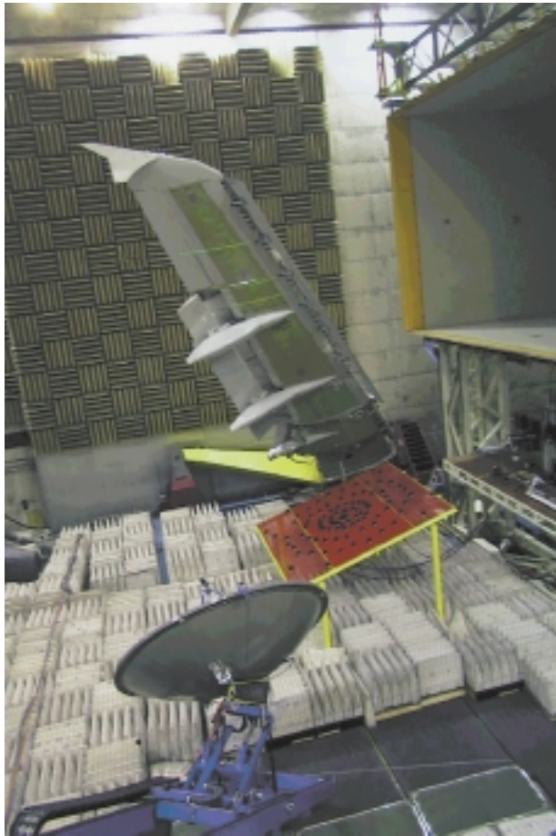
The identification of noise sources on a full-scale wing of an Airbus A320 is achieved with an acoustic mirror and a microphone array
