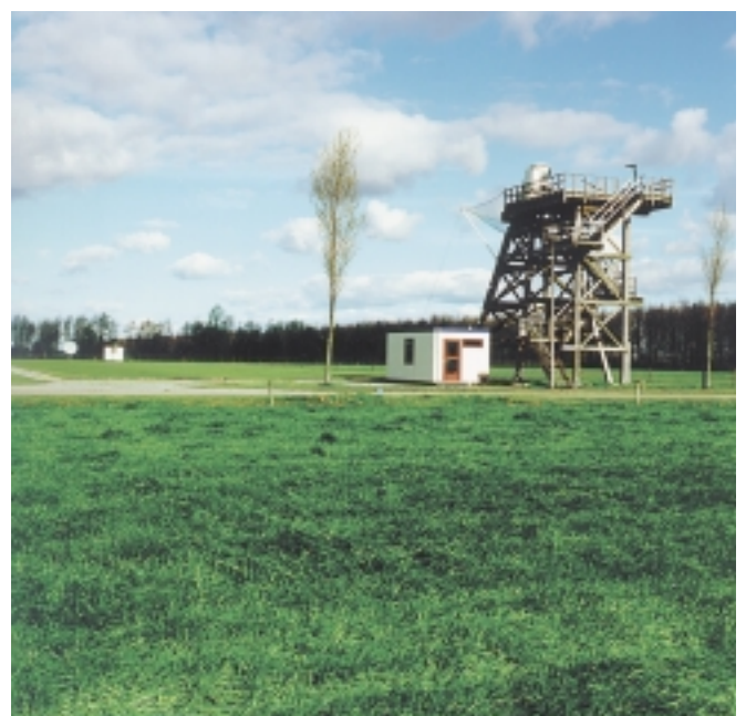
Outdoor Antenna Test Range, with a transmitter at 160m from the tower
