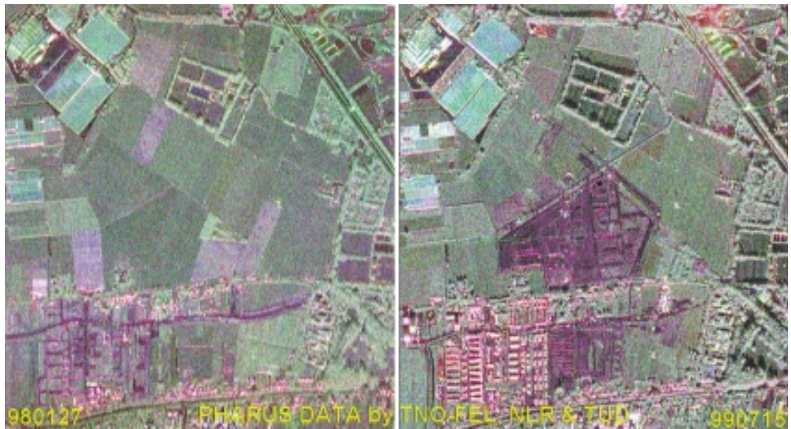
Two images of a region west of Utrecht made by PHARUS, a Synthetic Aperture Radar on the Citation II research aircraft, with differences between the left (older) and right image revealing building activities
