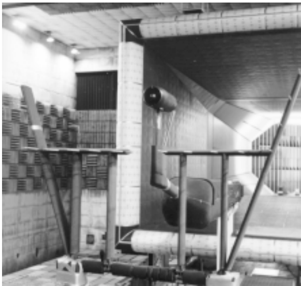
NLR's model turbofan in the anechoic open jet configuration of the DNW Large Low-speed Facility
