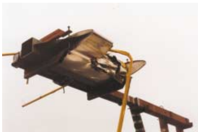
Fig. 9 – Impact test of a light aircraft wing section against a frangible approach light mast (courtesy Exel Oy)
