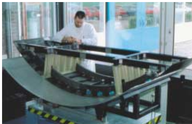
Fig. 8 – Composite energy-absorbing sub-floor structure for a commuter aircraft
