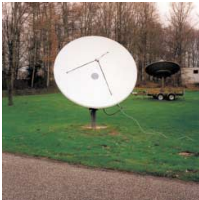
Antenna for dissemination of ERS data also capable of receiving transmissions from the Erasmus User Centre
