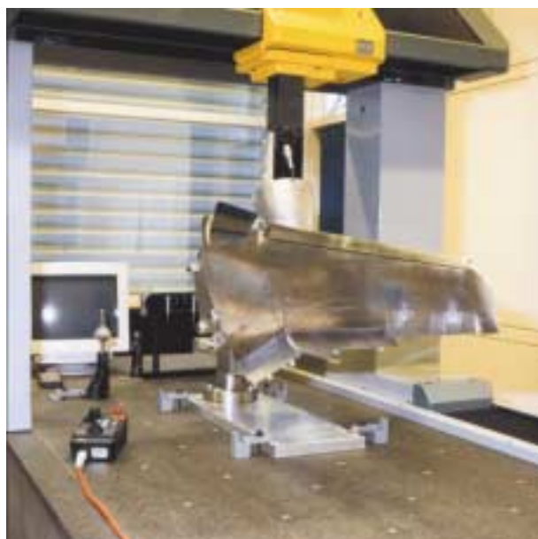
Wing of low-speed wind tunnel model on 3D co-ordinate measuring machine for geometry inspection
