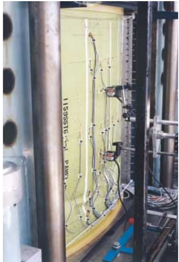
Shear test on fuselage panel of Gulfstream aircraft
