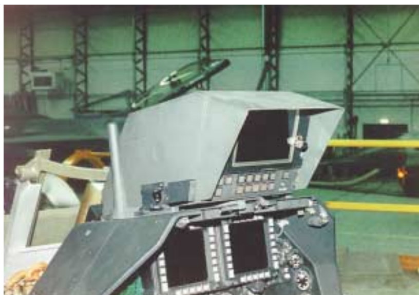
Aft seat HUD monitor console with instrumentation display
