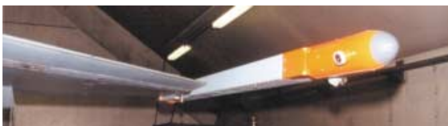
F-16 MLU Flight Test instrumentation: modified AMRAAM tip launcher with camera inside
