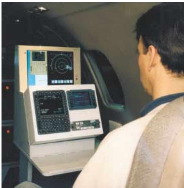
Navigation of the aircraft is done from the experimenter's station (shown) using datalink to communicate with simulated ATC
