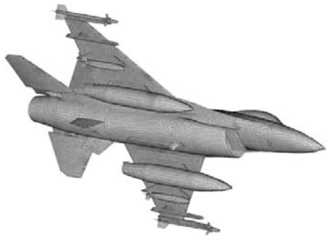
Computational surface grid on a fighter configuration for Radar Cross Section prediction
