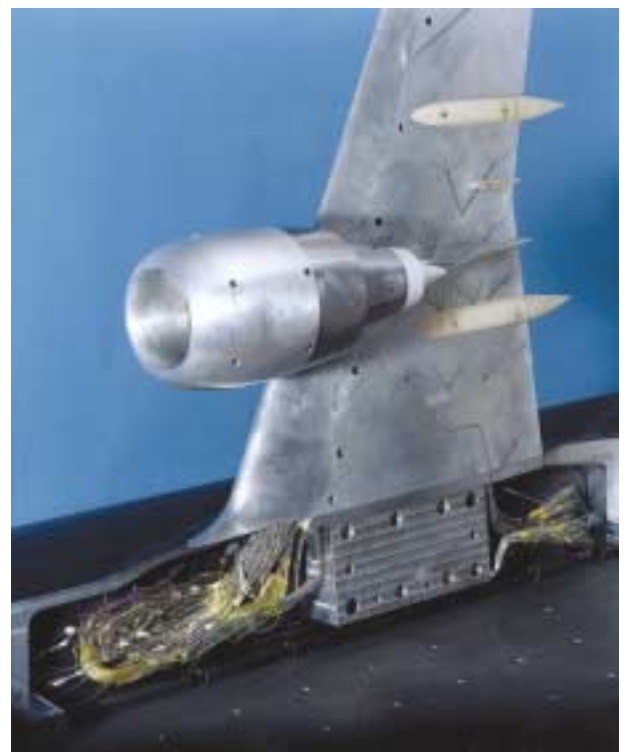
Wing with pressure instrumentation and nacelle with turbine powered simulator for high speed semi-span model
