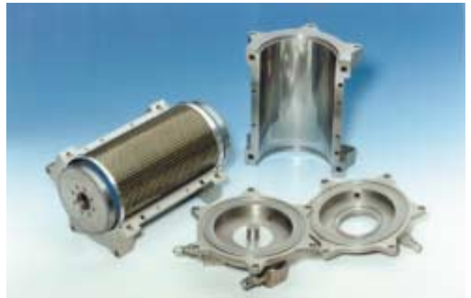
Fig. 4 – Crash tube for NH90 nose landing gear and fabrication tooling
