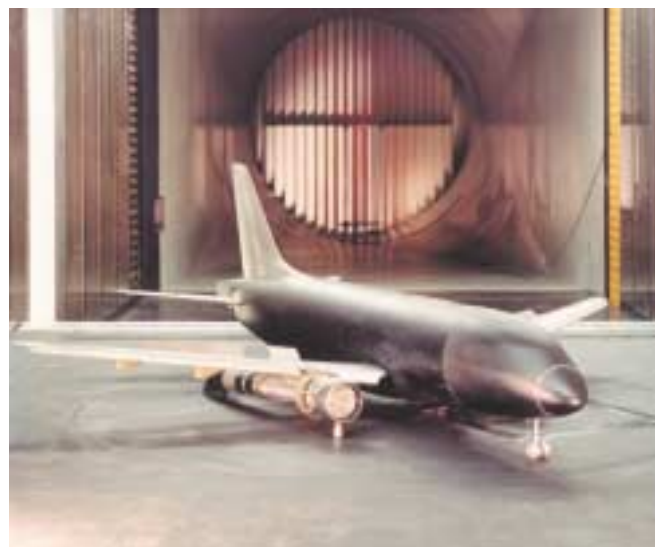
Fairchild Dornier model on ground board in the DNW-LST
