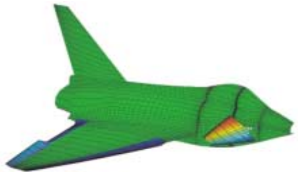
AESIM-BASIC surface grid around a modern fighter configuration
