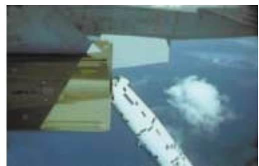
Separation of a fuel tank from an F-16 during navigation pod certification flight tests
