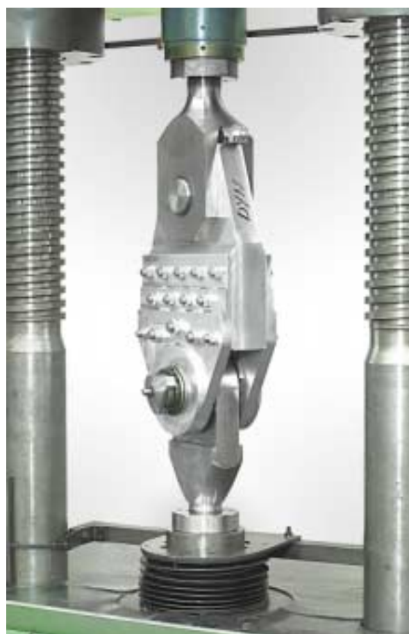
Fatigue test on fuse pin of Airbus A340 300/600 main landing gear
