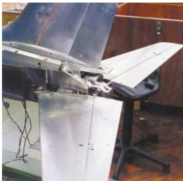
Tail section of low-speed wind tunnel model with remotely controlled elevator and rudder
