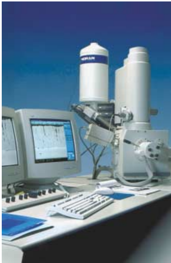
Field Emission Scanning electron microscope combined with energy dispersive material analysis equipment that became operational
