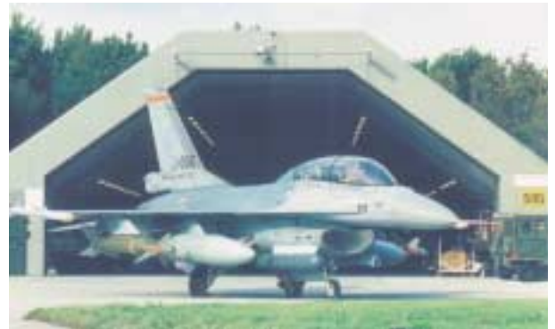
F-16 MLU test aircraft of the RNLAf equipped with navigation pod and targeting pod
