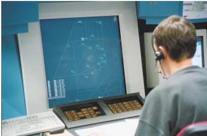
The real research aircraft is mixed with simulated air traffic; the real aircraft is controlled through datalink, using voice as backup
