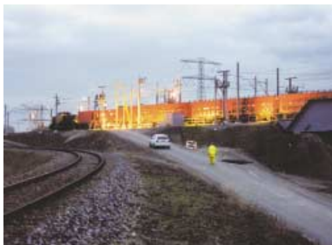
Instrumentation for testing high-voltage railway power supply system: static load train
