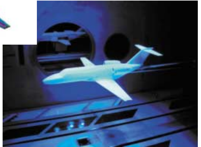
Boeing PSP (Pressure Sensitive Paint) method applied on a Cessna model in the DNW-HST (below), and typical results (top)
