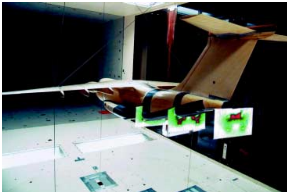
Fig. 2 – Particle Image Velocimetry measurements at three planes in the DNW-LST, for the A400M programme
