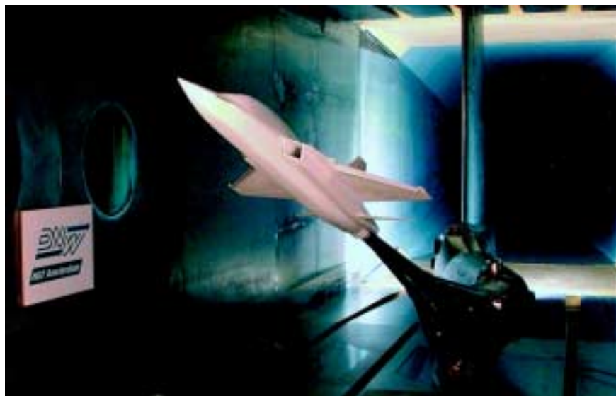
Fig. 4 – EADS Mako trainer model tested using Pressure Sensitive Paint in the DNW-HST
