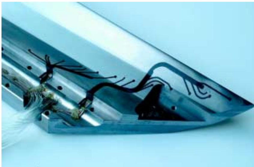
Detail of EPISTLE leading edge instrumented for pressure measurements
