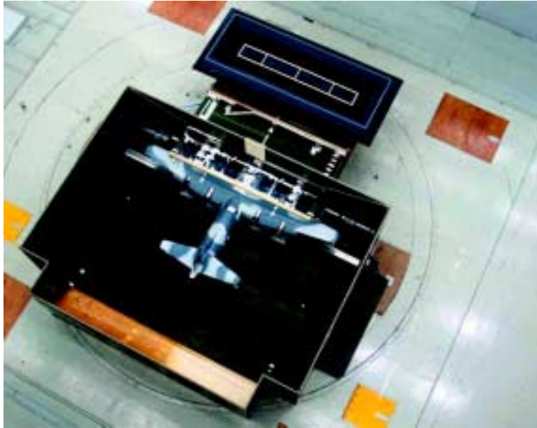
Wind tunnel set-up with full Ground Run-up Enclosure model and C-130 Hercules aircraft model
