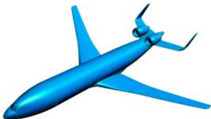
Low-noise aircraft configuration with exhaust jets shielded by tail surfaces
