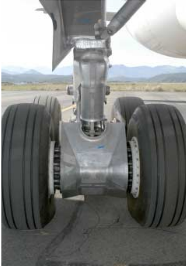
Main landing gear with noise-reducing streamline fairings tested in-flight in EU project SILENCE(R)
