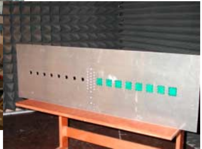
Aluminium plate with installed patch antennas for demonstrating smart phased array antenna.
