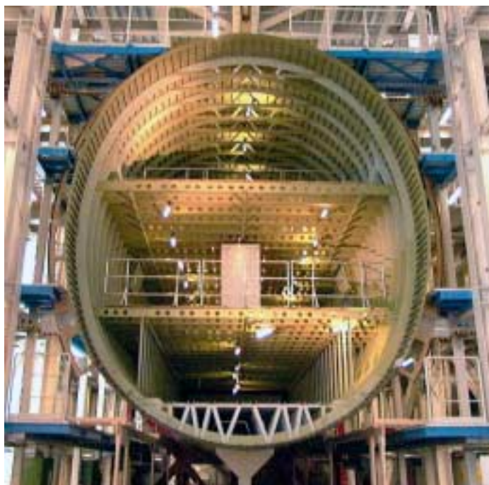
Fig. 8 An assembled barrel just before the mounting of the free pressure bulkhead
