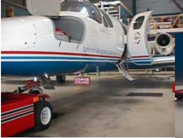
Structural modifications of the Citation (laser reflector of the Flight Inspection System) and the Chinook (missile warning system) that require vibration testing
