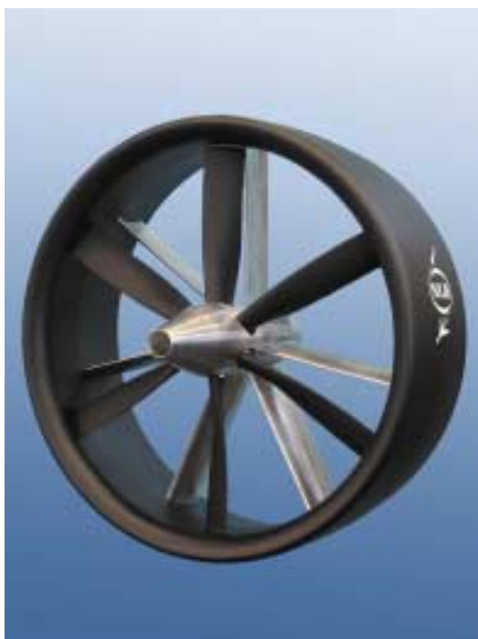
Wind tunnel model of ducted fan for hovercraft with six-bladed carbon fibre fan
