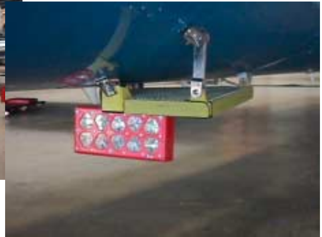
Structural modifications of the Citation (laser reflector of the Flight Inspection System) and the Chinook (missile warning system) that require vibration testing
