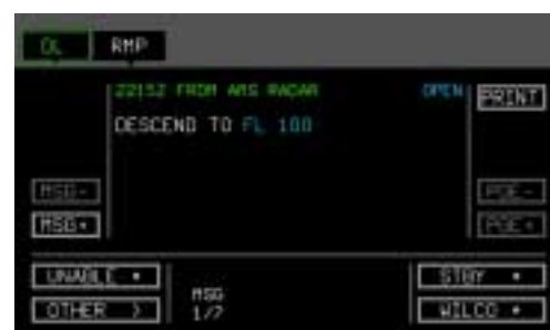
Figure 4 The new display units allow implementing new functions, such as datalink, in a natural way. Instead of installing a dedicated unit in the cockpit (top), the new function can be added to the display unit's software (bottom)
