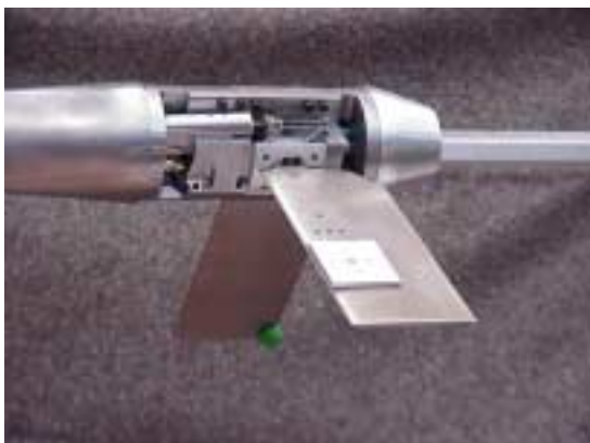
Transonic wind tunnel model of Air Refuelling Boom with remote control mechanism exposed
