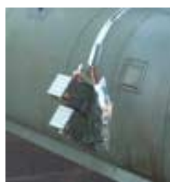
Structural modifications of the Chinook (missile warning system) that require vibration testing
