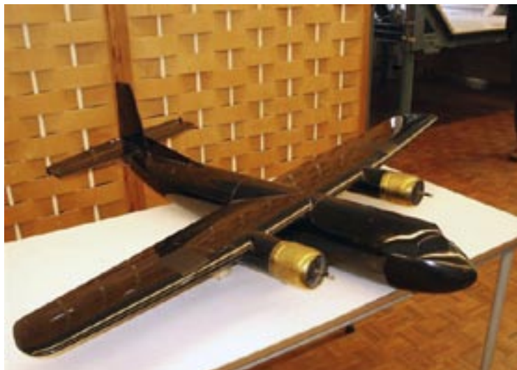
Fokker F.24 windtunnel model
