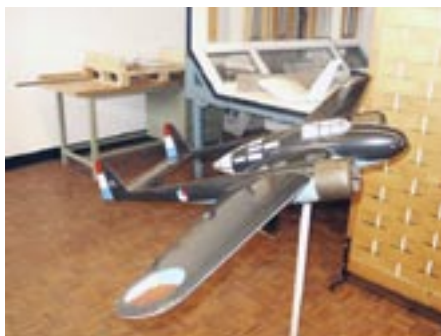
Fokker G-1 windtunnel model
