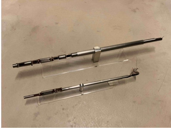
Figure 10 Two newly designed NLL sting-balances used in combination with the AGARD-C models in the Pilot Tunnel (1957).
